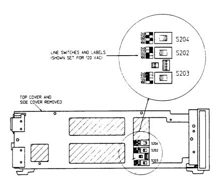
Figure 3-5. Line Voltage Switches
