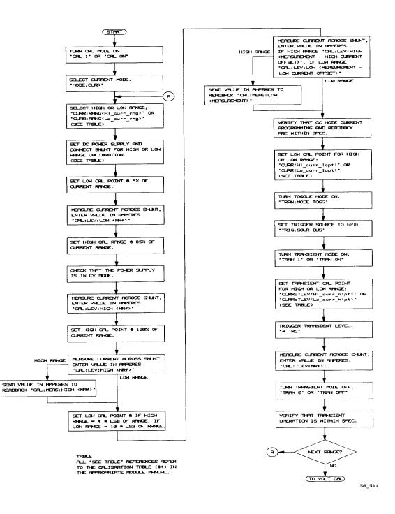
Figure 6-3. Calibration Flowchart for "B" Modules
