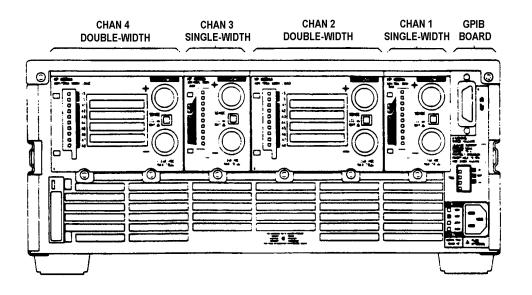
Figure 3-3. Channel Number Example (Agilent 6050A)
