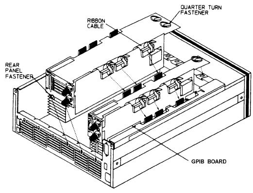
Figure 3-2. Limiting Modules In an Agilent
