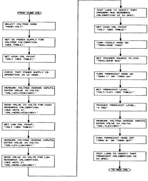
TRBLE FILL TRBLE REFERENCES REFER TO THE CALIBRATION TRBLE IN THE MODULE MANURL. NOTE 2 REFIDERCK DIAC DOES NOT NECESSARILY HAVE TO BE CALIERATED TO THE SAME ACCURRCY AS THE PROGRAM DIAC.
