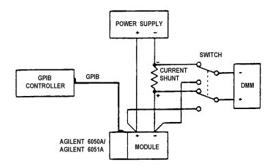
Figure 6-1. Calibration Equipment Setup
