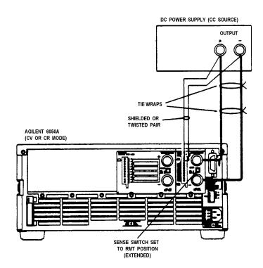
Figure 3-13. Remote Sensing
