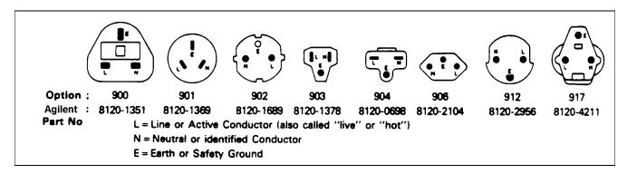
Figure 3-1. Power Cord Configurations
