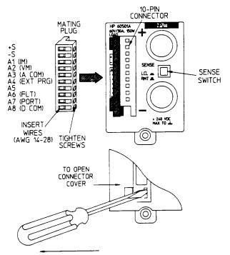
Figure 3-10. Control Connector and Cover
