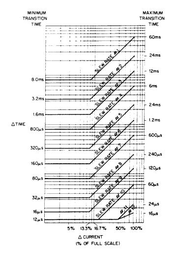
Figure 2-9. Transition Times and Slew Rates
