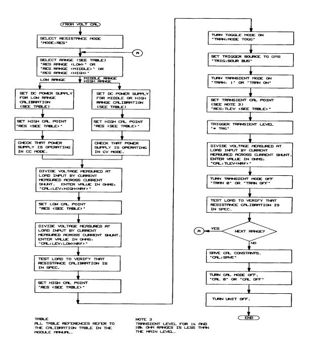
Figure 6-2. Calibration Flowchart for "A" Modules (continued)
