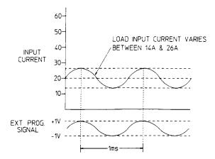
Figure 2-10. External Programming Example
