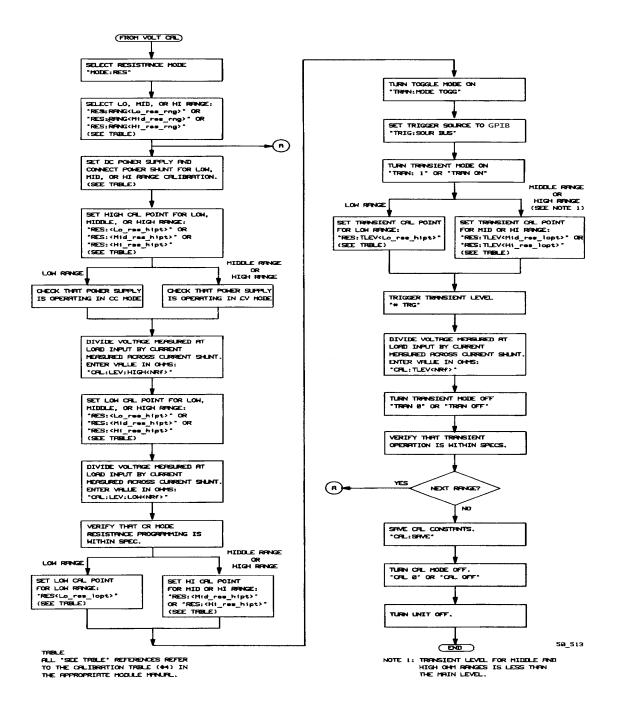
Figure 6-3. Calibration Flowchart for "B" Modules (continued)
