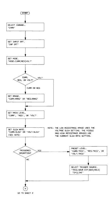
Figure 5-1. Remote Programming Flowchart (Sheet 1)
