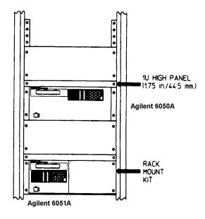
Figure 3-4. Rack Installation
