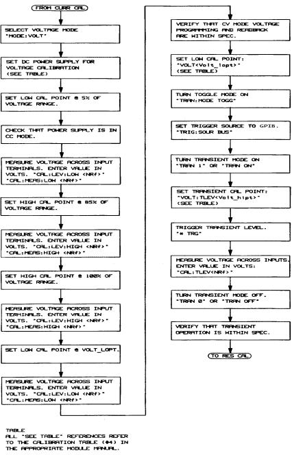
Figure 6-3. Calibration Flowchart for "B" Modules (continued)
